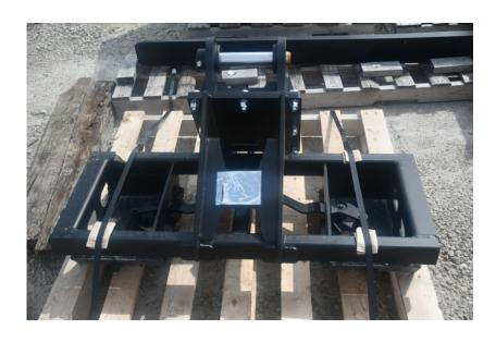
Attachments: 2020 AMI Kobelco SK85 to Skid Loader
