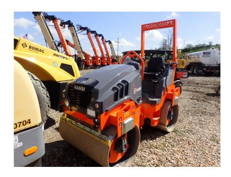
Compaction Equipment - Smooth Drum: 2019 Hamm HD12VV Smooth
