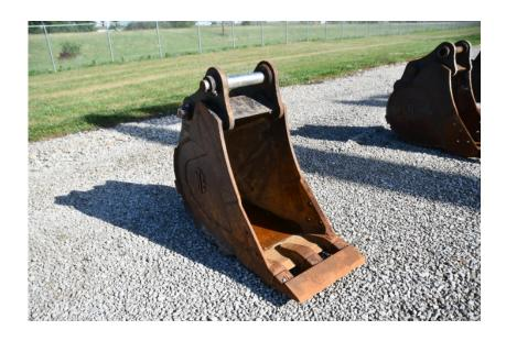
Attachments: TAG 24" SK210/SK235SR/SK230SR/SK270SR Excavator
