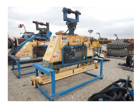
Attachment Surplus: 2012 Vacuworx MC5 Steel Pipe Lifter
