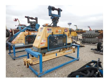
Misc: 2012 Vacuworx MC5 Steel Pipe Lifter
