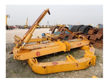
Attachments: Rockland D6T LGP Angle Blade and C Frame
