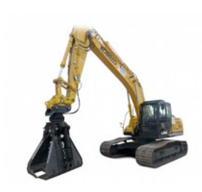
Excavators W/mat Grapples: EXCAVATORS WITH MAT GRAPPLES
