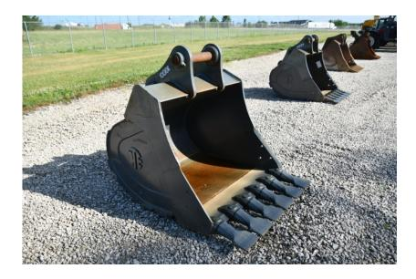
Attachments: TAG 48" SK210/SK235SR/SK230SR/SK270SR Excavator
