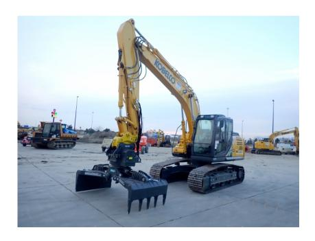
Excavator: 2021 Kobelco SK170LC-10 w/Heavy Counterweight
