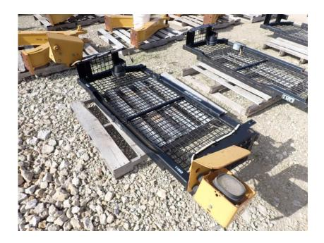
Attachments: CAT D8T Rear Window Cab Protection Screen Stock Number: JT010
