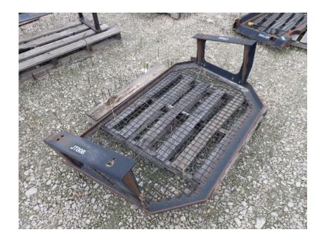
Attachment Surplus: CAT D6T Rear Window Cab Protection Screen Stock Number: JT008SUR
